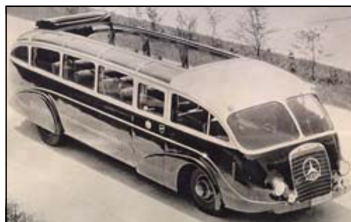
Mercedes omnibus with curved Plexiglas roof lights (1937).
