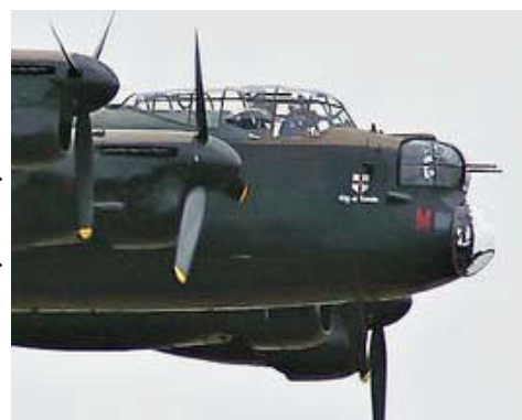
Royal Air Force Avro Lancaster bomber with nose cupola and other glazing made from Perspex.
